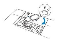
Insert the tabs on the needle plate cover into the needle plate, and then slide the cover back on.
