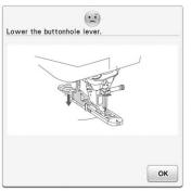
This message is displayed when the buttonhole lever is up, a buttonhole stitch is selected, and the "Start/ Stop" button or "Reverse/ Reinforcement Stitch" button is pushed.
