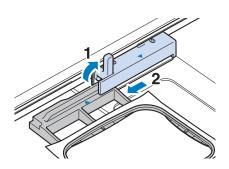
Insert a wound bobbin into the machine. (see page 59 for Setting the bobbin.)
