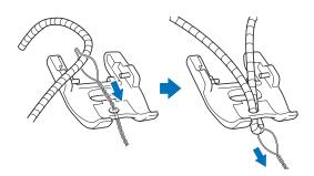
Attach the toe of the couching dual feed foot shown below to the dual feed foot.
