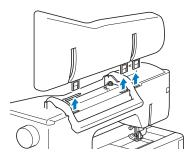
Insert the spool stand onto the notches of the machine.
