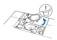
Set the straight stitch needle plate in place and use the multi-purpose screwdriver to tighten the plate.
