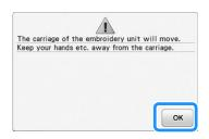
→ The built-in camera automatically searches for the embroidery positioning sticker, and then the carriage is moved so that the selected reference point of the embroidery pattern is aligned with the embroidery positioning sticker. The brightness of the machine light is dimmed while the built-in camera searches for the embroidery positioning sticker.
