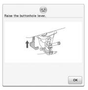
This message is displayed when the buttonhole lever is down, a stitch other than a buttonhole is selected, and the "Start/ Stop" button or the "Reverse/ Reinforcement Stitch" button is pushed.
