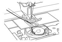
Install the needle plate cover and bobbin cover with tabs.
