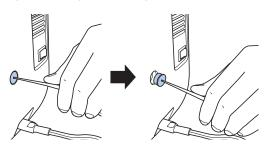
Firmly insert the sensor pen holder into the hole where the protective cap was removed.
