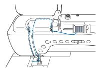
Pass the thread through the needle bar thread guides on the needle bar, then thread the needle on the left side manually.
