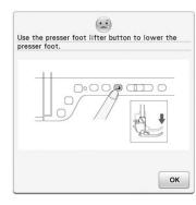
This message is displayed when a button, such as the "Start/Stop" button, is pushed while the presser foot is raised.
