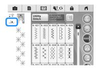
→ The machine automatically stops with the needle in the fabric, at about half the distance to the specified sewing end point, and the sewing end point setting screen appears.
