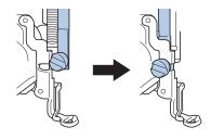
Hold the embroidery foot in place with your right hand, and then use the included multi-purpose screwdriver to securely tighten the presser foot holder screw.
