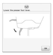
This message is displayed when the "Presser Foot Lifter" button is pushed while the presser foot lever is raised/the needle is lowered.
