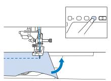
The pivot setting is useful when changing the sewing direction. When the machine is stopped at the corner of the fabric, the machine stops with the needle in the fabric and the presser foot is automatically raised so the fabric can easily be rotated ("Pivoting" on page 95).
