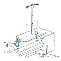
Place the spool of thread on the spool pin so that the thread feeds off the spool clockwise. Firmly insert the spool cap onto the spool pin.
