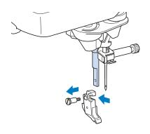
Set the adapter on the presser foot bar, aligning the flat side of the adapter opening with the flat side of the presser bar. Push it up as far as possible, and then tighten the screw securely with the screwdriver.
