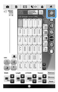
→ The key appears as , the quilting foot is raised to the necessary height, and then the feed dogs are lowered for free motion sewing.
