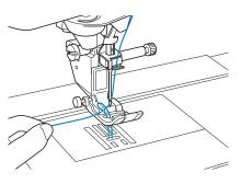
Pull up the bobbin thread, pass it under the presser foot and pull it about 100 mm (approx. 3-4 inches) toward the back of the machine, making it even with the upper thread.
