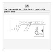
This message is displayed when the embroidery unit is attached and the power is turned on with the needle in the down position.
