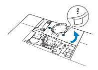
Use the cleaning brush or a vacuum cleaner to remove any lint and dust from the cutter in the bobbin case area.
