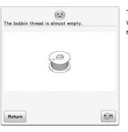
This message is displayed when the bobbin thread is running out.
