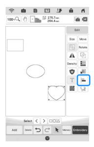
Touch each pattern to select multiple patterns and then select the key for the desired alignment.
