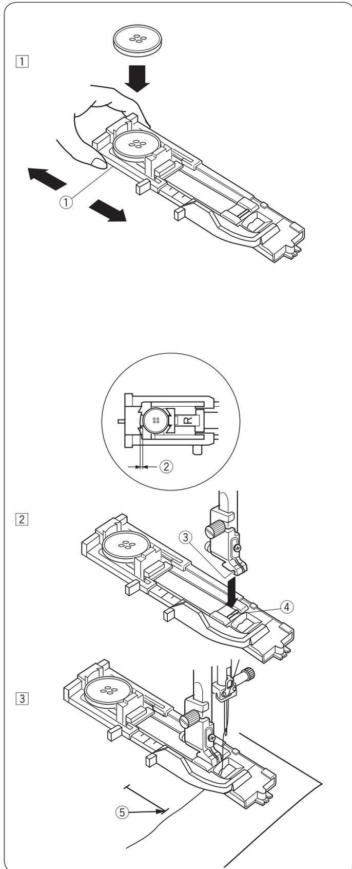
The size of a buttonhole is automatically set by placing a button in the rear of automatic buttonhole foot R. The button holder of the foot takes a button size of 1 cm (3/8") to 2.5 cm (1") in diameter. When selecting the buttonholes, the LCD screen advise you to lower the buttonhole lever.
