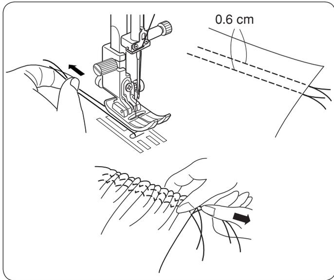
Loosen the thread tension to “1” and increase the stitch length to 5.0.
