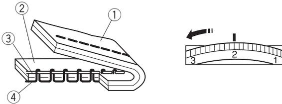
Turn the thread tension dial to a lower number to decrease the thread tension.
