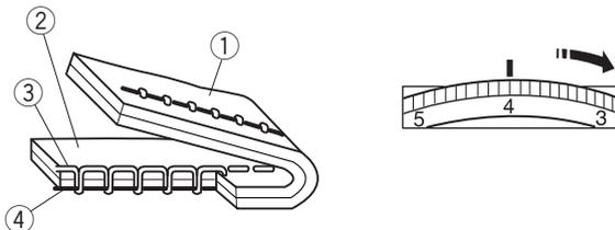
Turn the thread tension dial to a higher number to increase the thread tension.
