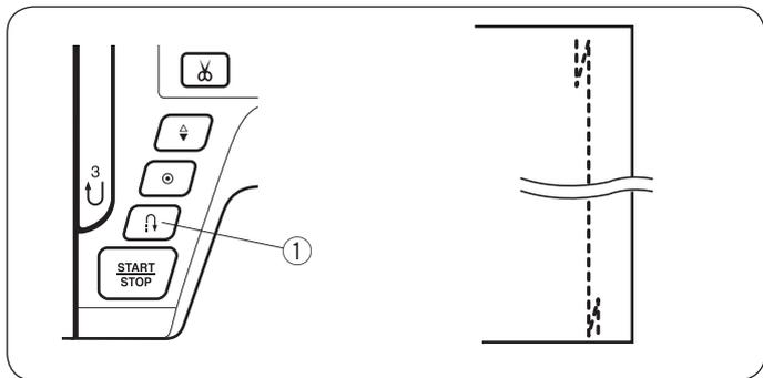
Use this stitch to secure the beginning and the end of a seam with backstitching. When you reach the end of the seam, press the reverse button ① once. The machine will sew four reverse stitches, four forward stitches, and then stop sewing automatically.
