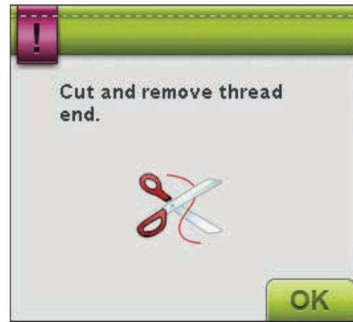
7. When the first color is completed, your machine cuts the thread end and stops. A pop-up message appears asking you to change thread color. Re-thread with the next color and continue embroidering by pressing Start/Stop. Hold the thread end. The machine will trim the top thread and pull the thread to the underside of the fabric.
