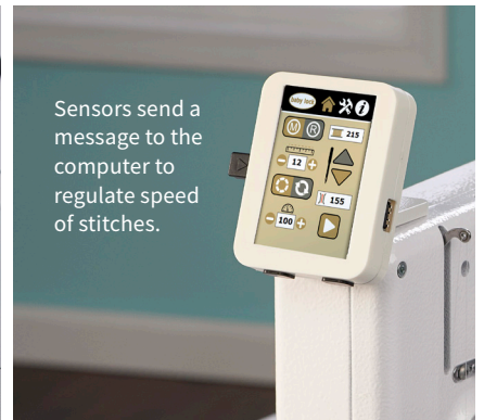
Sensors detect fabric motion speed.
