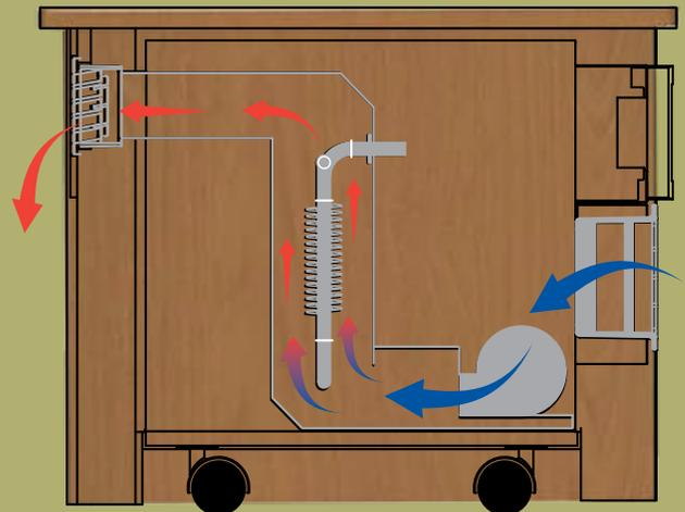
With SewComfort Heaters, air is drawn from the floor level through a washable lifetime filter. This filtered air then enters the heating chamber, passes through an exclusive mineral-filled tubular heating element, and then out of the heater through a specially-designed front louvered grill.
