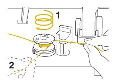
**B** Pass the end of the thread through the guide slit in the bobbin winder seat, and pull the thread to the right to cut the thread with the cutter.
