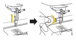
**5** Insert the included small screw into the threaded hole in the adapter and turn it 2 or 3 times with your hand.
