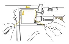
B Guide the thread down, up, then down through the groove, as shown in the illustration.
