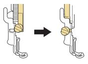
Hold the embroidery foot in place with your right hand, and then use the included screwdriver to securely tighten the presser foot holder screw.
