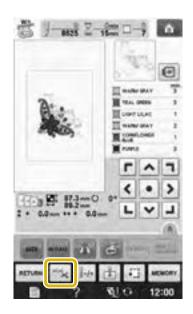
Press **m** to turn off the automatic thread cutting function.
