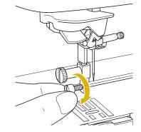
Set the operation lever of the walking foot so that the needle clamp screw is set between the forks. Position the shank of the walking foot on the adapter attached to the presser foot bar.
