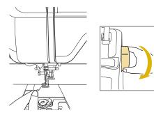
Gently pull the upper thread to bring the bobbin thread up through the needle plate.
