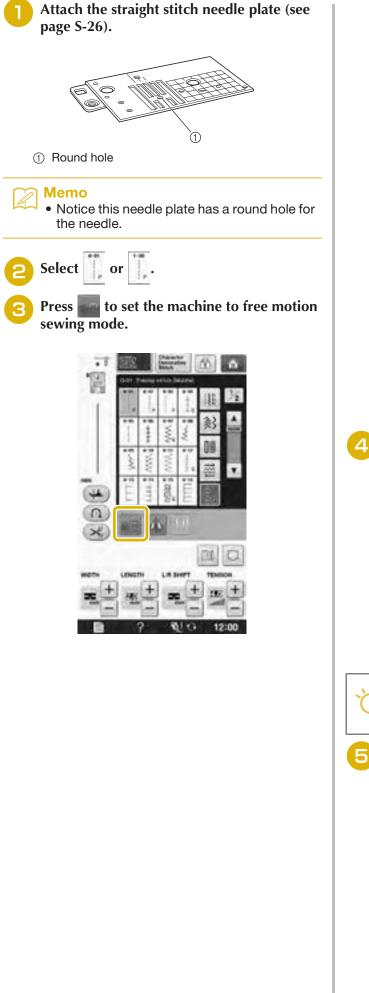
$\rightarrow$  The key appears as **\overline{}**, the quilting foot is raised to the necessary height, and then the feed dogs are lowered for free motion sewing.
