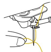
**15** Raise the presser foot lever and pull out about 10 cm (approx. 4 inches) of the thread, and then pass it under the presser foot toward the rear of the machine.
