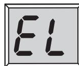
*Note: During the sewing, if the thread get jammed inside the hook stopping the needle from moving and you continue pressing the foot control, the security switch will stop the machine completely. In order to restart the sewing machine, you will have to turn the ON/OFF switch to the OFF position and then ON again.*
