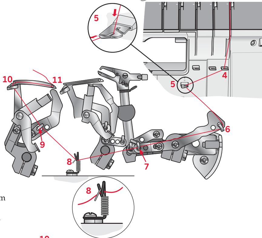
*Tip: Moving the stitch finger lever to R makes the threading easier. Remember to set it back to N before starting to sew.*
