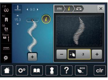
To correct the longitudinal direction of the stitch pattern, turn the «Lower Multi-function knob» until the > preview of the stitch pattern matches the stitch pattern sewn on the fabric.
