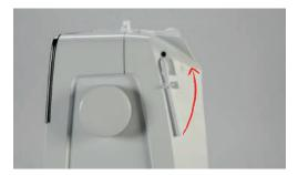
Inserting foam pad and thread spool The foam pad prevents the thread from getting hooked at the swiveling spool holder.
