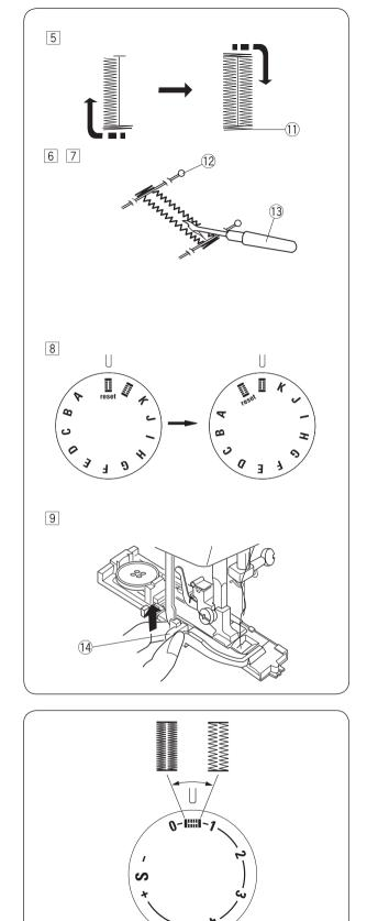
Depress the foot control to sew a buttonhole. The machine automatically sews the front bartack, the left row, the rear bartack and the right row. Stop the machine at the ending point.
