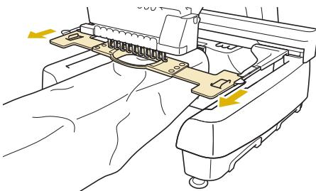
**2** Hold the handle at the bottom of the tubular frame table and return the extended tubular frame table to its original position.
