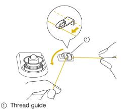
6 Pass the thread around the pretension disk making sure that the thread is under the pretension disk.
