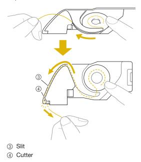
Sewing with the correct thread tension is possible after the bobbin has been correctly installed in the bobbin case.
