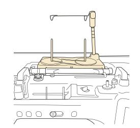
Place the spool of thread on the spool pin so that the thread feeds off the spool clockwise. Firmly insert the spool cap onto the spool pin.
