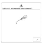
Once this message appears, it is recommended to take your machine to an authorized Baby Lock retailer for a regular maintenance check. Although this message will disappear and the machine will continue to function once you press or, the message will display several more times until the appropriate maintenance is performed.
