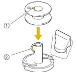
Pivot the spool pin so that it angles upward. Set the thread spool on the spool pin so that the thread unwinds from the front of the
