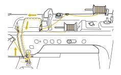
Continue threading; however, do not pass the thread in the needle bar thread guide "6" on the needle bar. Thread the needle on the right side.
