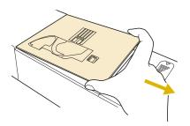
Insert the tabs on the straight stitch needle plate into the notches in the machine.
