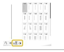
Place the fabric under the presser foot with the needle at the starting point of the stitching, and then press the "Start/Stop" button. The machine will begin sewing.
