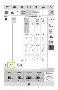
$\rightarrow$  You get  $\widehat{\Box} \gg$ , and the machine is set for automatic thread cutting function and automatic reverse/reinforcement stitching.
