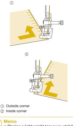
Placing a lightweight tear away stabilizer beneath the stitching area will improve the stitch placement along the edge of the appliqué fabric.
