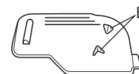
Bobbin cover There are two small v-shaped tabs on the back of the bobbin cover as indicated by the letter "B". The tabs help hold the bobbin in place so it does not lift up while thick thread is being pulled through.
