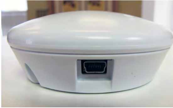
Figure 4. USB Mini-B style charging port on the Controller.
