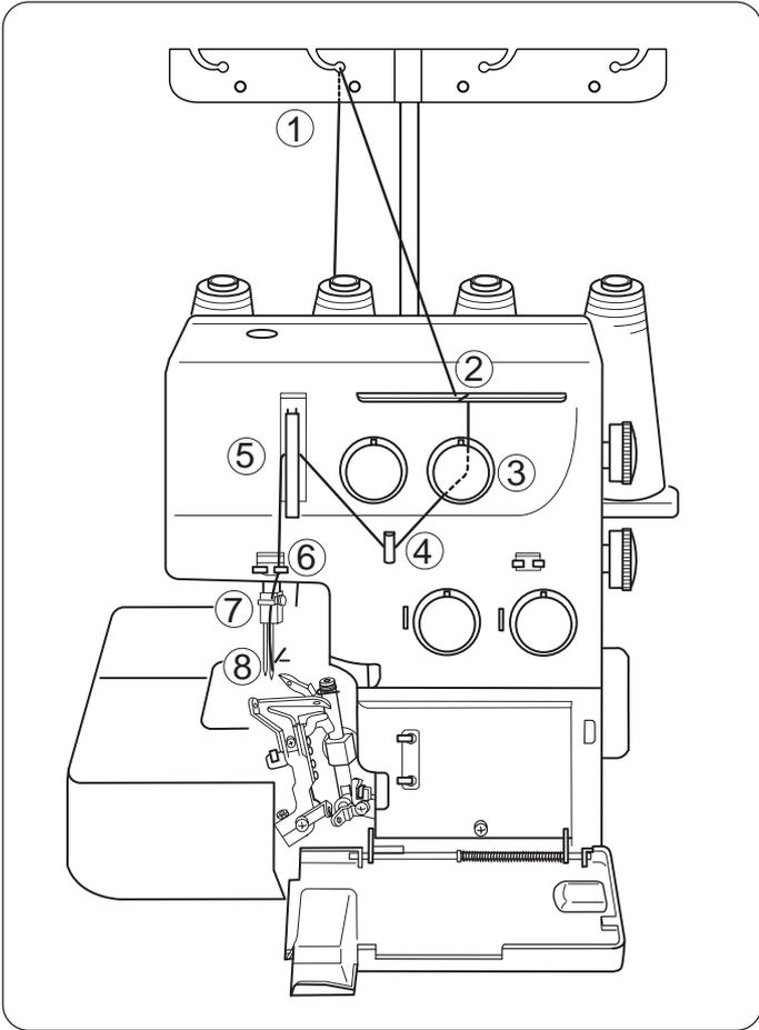
1. Draw the thread through the thread guide second from the left from back to front: (A)
