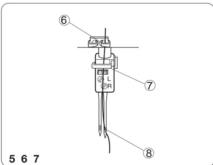
5. Pass the thread through the needle thread guide sliding the thread from left to right.
