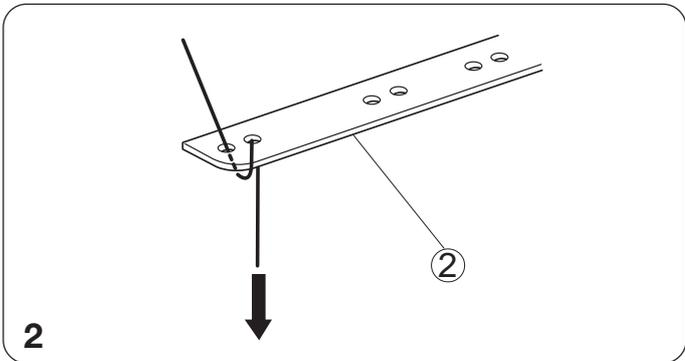
2. Pass the thread through the holes on the left of thread guide plate as illustrated.
