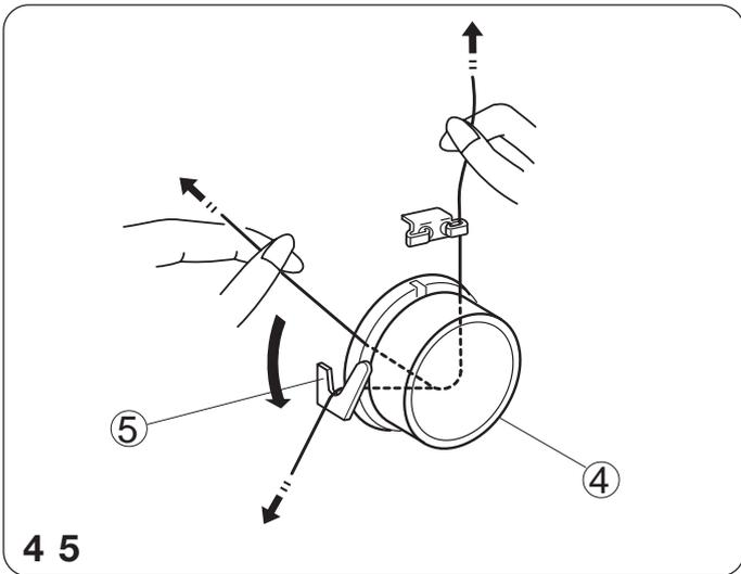
4. Insert the thread between tension discs from the right. Then pull both sides of the thread firmly to insert it between tension discs.
