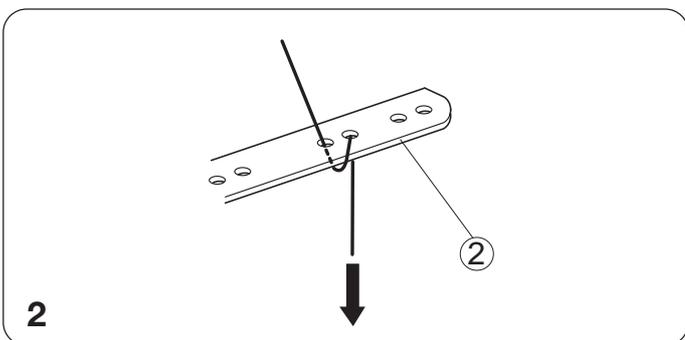
3. Pass the thread through the left side of looper thread guide sliding the thread from right to left.
