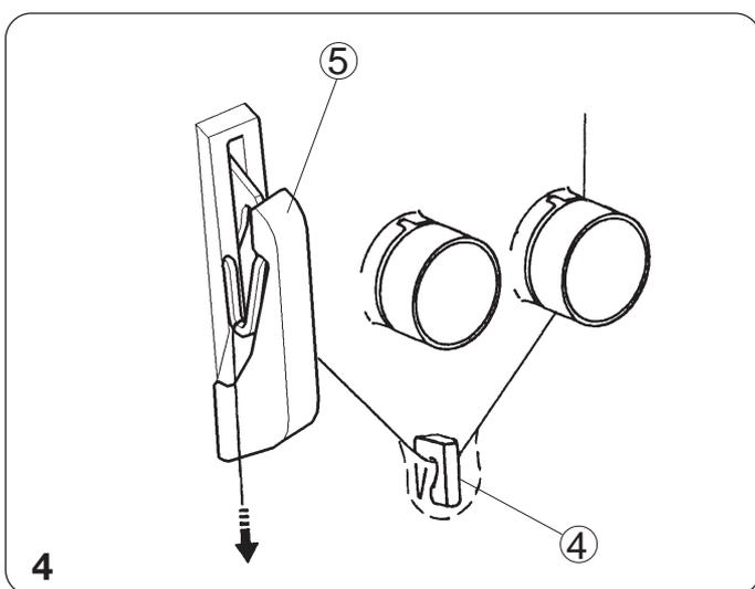
4. Turn the handwheel toward you to bring the needle bar to its highest position, then pass the thread through the right needle thread guide and the thread take-up lever cover.
