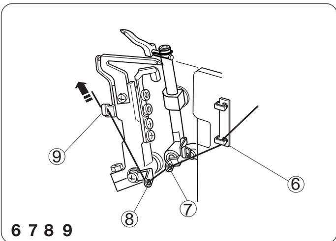
6. Pass the thread through lower looper thread guide (2).
