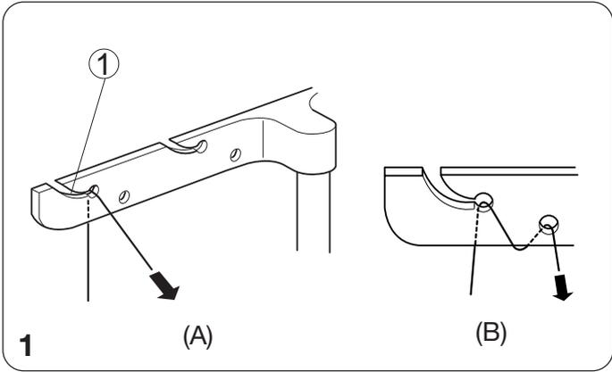
1. Draw the thread through the thread guide on the left from back to front: (A)
