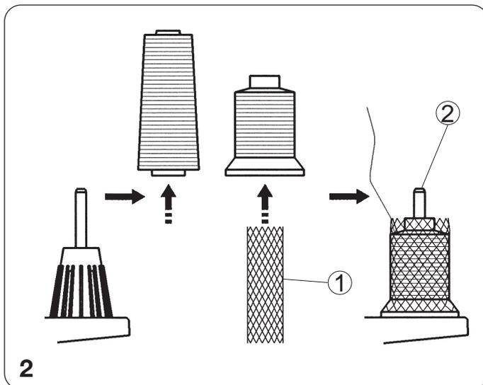
2. If the thread slips down from the spool during threading and/or sewing, put a net on the spool as illustrated to prevent jamming.
