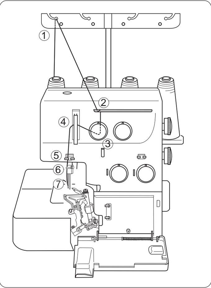
• **Threading the Needle on the Left**
