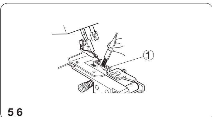
5. Brush out the lint around the feed dogs to the front by using the lint brush or use a vacuum cleaner.
