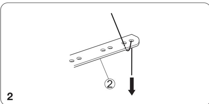
2. Pass the thread through the holes on the right side of the thread guide plate as illustrated.
