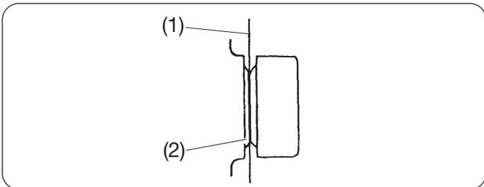
\* Make sure that the thread is between the tension discs.
