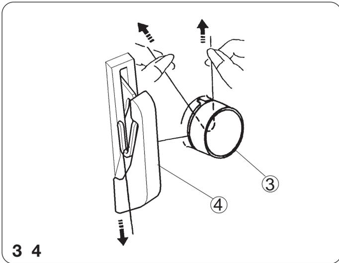
3. Insert the thread between tension discs from the right. Then pull both sides of thread.
