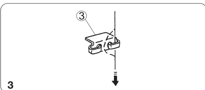
3. Pass the thread through the right side of the looper thread guide, sliding the thread from left to right.
