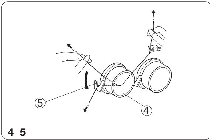
4. Insert the thread between tension discs from the right. Then pull both sides of thread.
