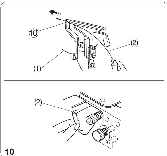
10. Turn the handwheel toward you until the lower looper comes to the right, and pass the threader through the hole on lower looper thread guide (5).
