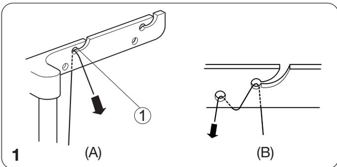
2. Pass the thread through the holes in the second row from the right of thread guide plate as illustrated.
