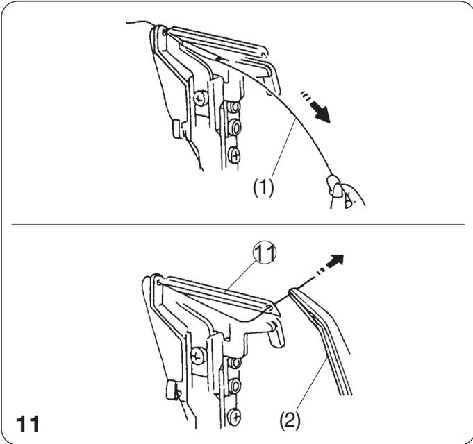
11. Pull the threader to pass the thread through the hole of lower looper thread guide (5).
