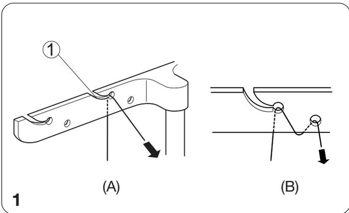
2. Pass the thread through the holes in the second row from the left of the thread guide plate as illustrated.
