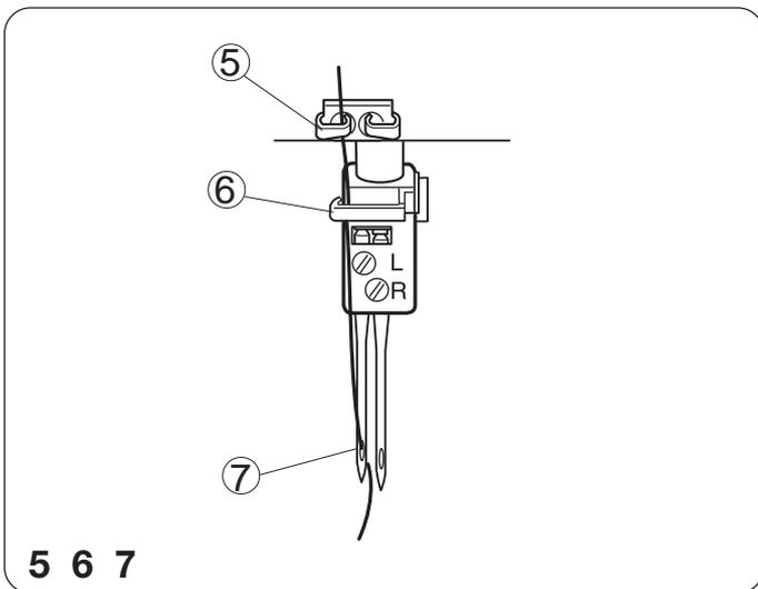
5. Pass the thread through the needle thread guide sliding the thread from right to left.
