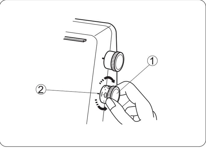
**Adjustment of Differential Feed Ratio**
