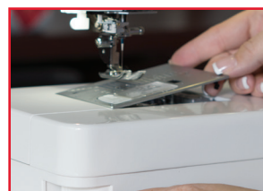
One-Step Needle Plate Conversion
