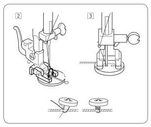
2 Match the holes in the button with the horizontal slot on the presser foot.
