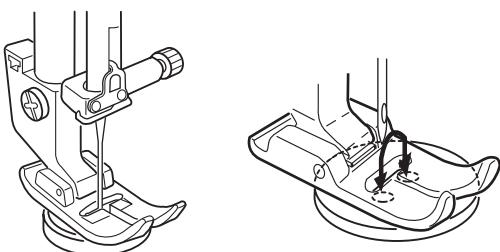
Unthread the needle. Adjust the stitch width to match it with the span of the holes in the button. Turn the handwheel to check if the needle enters into each hole in the button.
