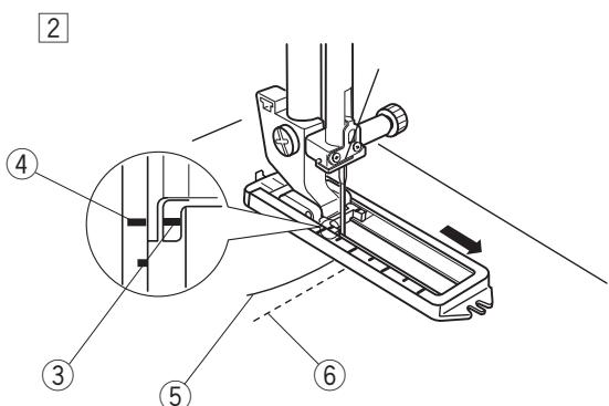
Draw both of needle and bobbin thread to the left. Move the slider toward you so that the top mark ④ on the slider meets the start arrow ③.
