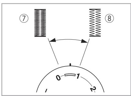
① Set the pattern selector dial at “”. Carefully mark buttonhole length on fabric. Place the fabric under the foot with the buttonhole marking running toward you.
