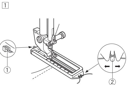
With the buttonhole foot raised, hook the filler cord on the spur at the back of the foot.
