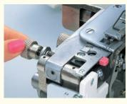
ADJUSTABLE CUTTING WIDTH Depending on the type or thickness of the material you sew, the seams may be too loose or too tight even when the tensions are correctly adjusted. In these cases, you can easily adjust the cutting width with this dial to correct the seam tension.
