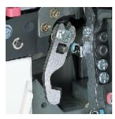
Upper knife can be quickly and easily deactivated by the turn of a knob.
