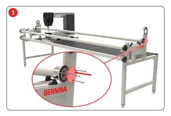
> Tighten the cover with 3 screws.
