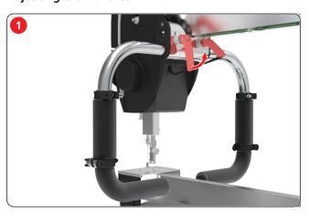
> Loosen the locking levers on both sides.
