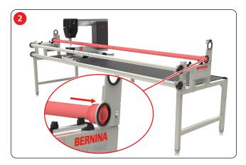
> Slide the right end of the rail through the the lower right rail holder.
