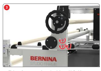
> Tighten 3 screws each on the right and left sides.
